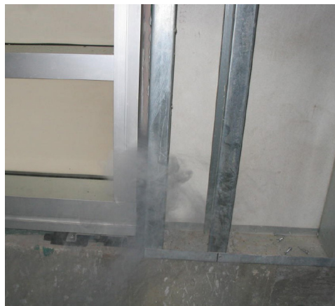
Using theatrical smoke under pressure makes air leakage visible and serves as a diagnostic tool.
