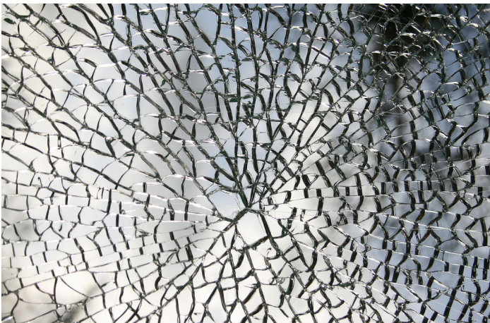
From top: two examples of glass edge damage (top image courtesy Bruening Glass Works); tempered glass breakage - note the glass remains within the frame; possible inclusion break identified by "butterfly-wing" break pattern at center; Right: microscopic nickel sulfide inclusion
