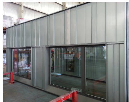
Above and left: Panelized wall detail: unit A (red) is inserted into the sill section (blue); pre-fabricated glazing assembly incorporated into a panelized exterior wall assembly; exterior wall panel staged at the site for erection
