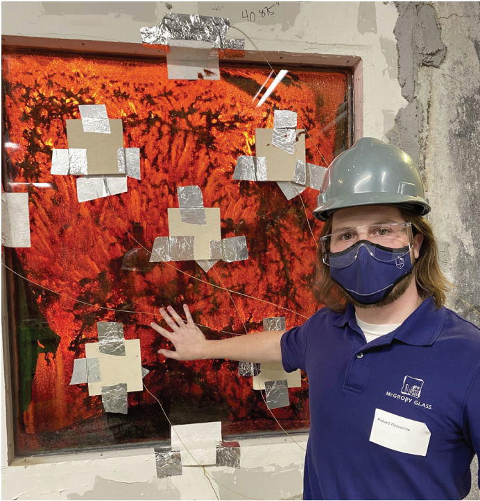
Left: Richard Whitcombe participating in a fire rating test, demonstrating the ability to touch the glazed surface even when subject to intense heat; right: click to watch a demonstration of how the butt-glazed AGC Vision Line glass partitions go together at the DHI Connexions Conference in October.
